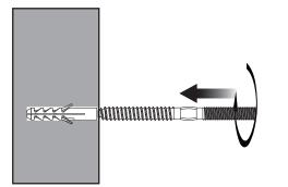
3.Screw a fixing bolt into each fixing plug using a 8mm spanner until the spanner contacts the wall
