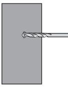
1.Drill two holes in the required position on the wall using a 14mm masonry drill bit.to a depth of 75mm
